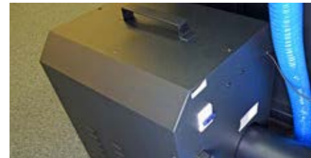
Acoustically housed, high pressure vacuum fan
